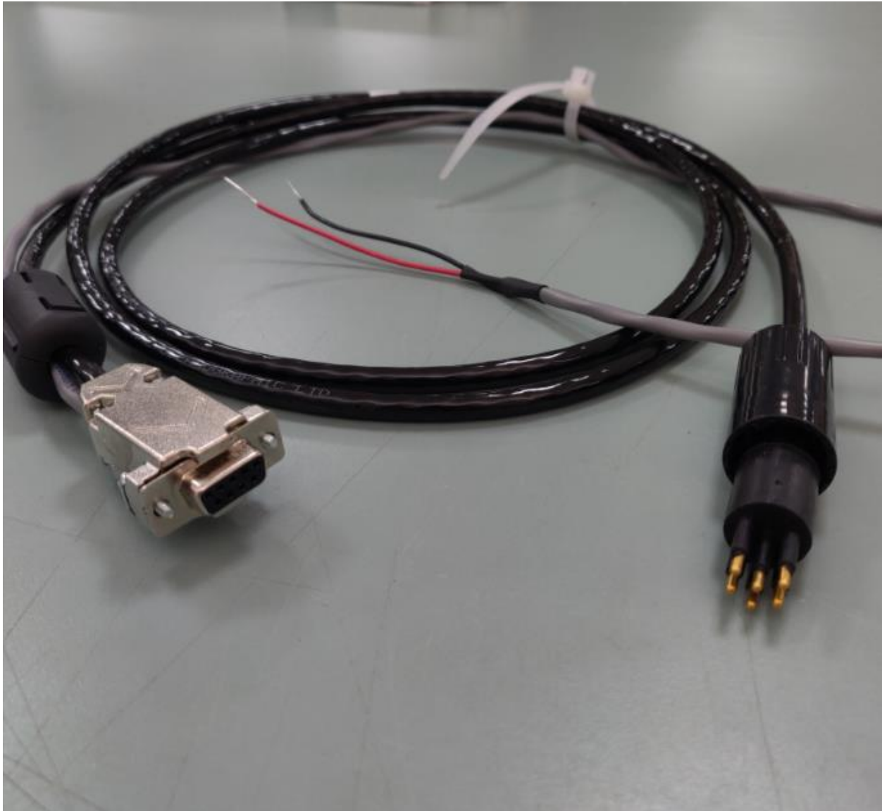
Figure 3. Waterproof cable (black) connected between the AML-1 RT and an RS232 port of the AMOS computer. The grey cable supplies power (red +12 V and black GND) to the black cable and the AML-1 RT.
